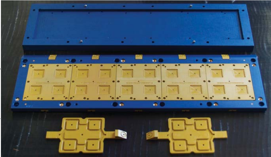
FIGURE 5. A strip testing socket with thermal management.
